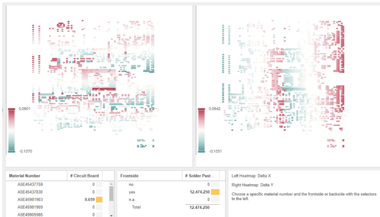
Fig. 5: A localized visualization of the parameters based on the position of the component on the board was found to be very helpful. A corresponding 'heat map' display was integrated into the functionality of the Causal AI solution.
